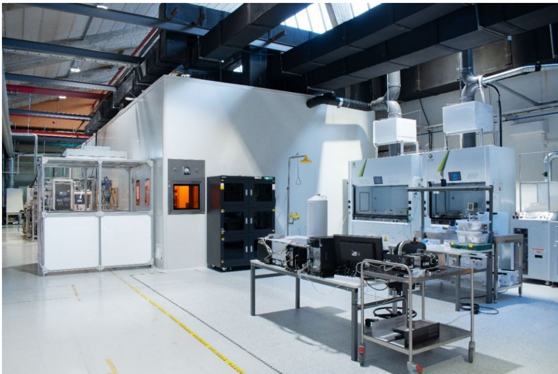
Figure 1 Exterior view of Comptek Solutions' new ISO cleanroom facilities, showing the pilot line and external chemistry process station
